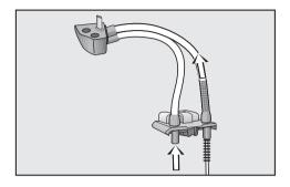
■ Push the brush into both milk pipes from below. Move the brush in and out of the pipes as far as it will go until there are no milk residues left in them.
